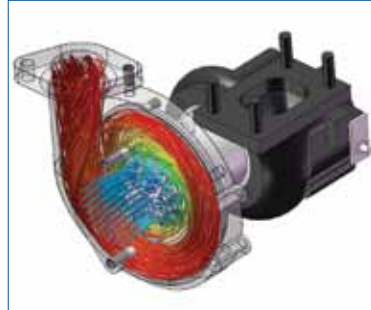
FloEFD can show the visual results of 'Flow Field' analysis in several formats; shown here as stream lines that can be tracked from point of origin to point of exit
